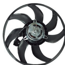
Palio 51285OM // Palio Diesel / TD 1,7 2001=> c./aire acond. s/Encauza- dor Ø39cm. Terminales 2.
