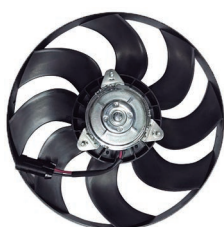
Boxer / Jumper 50809 // Boxer 2,3 2009=> (principal) / Jumper s/Encauzado Ø37 cm. Terminales 2.
